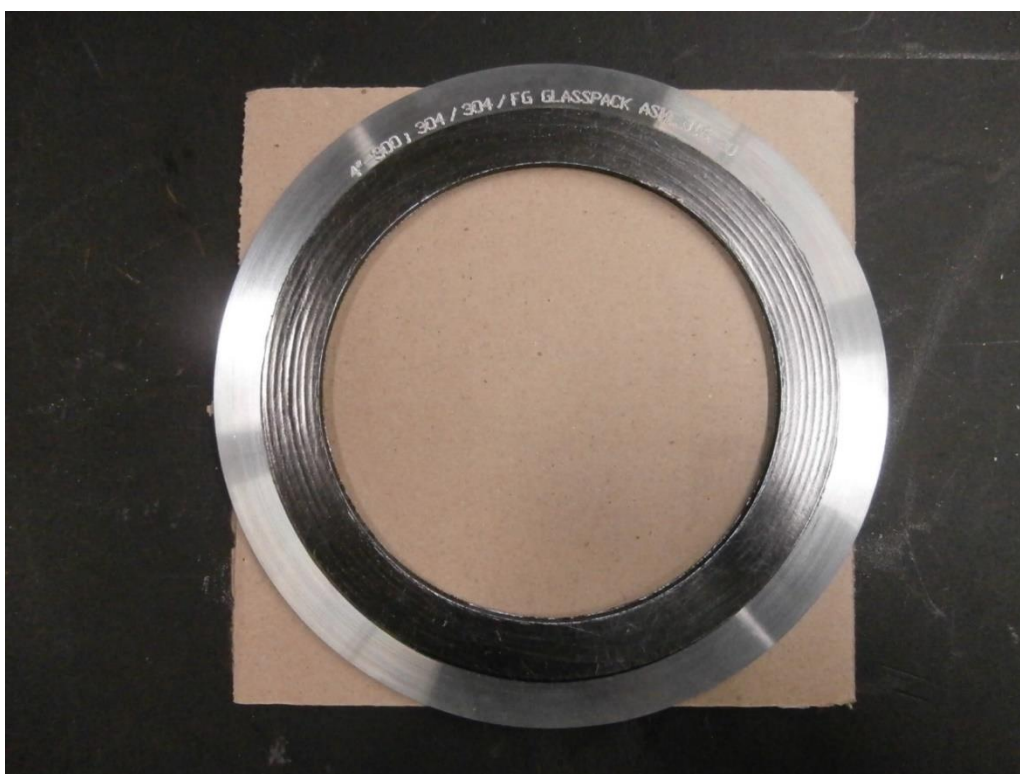
Test Gasket Prior to Test
